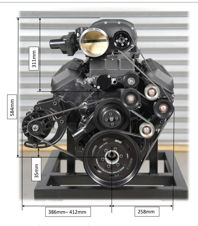
584mm C/L OF CRANK TO TOP OF S/C 311mm TOP OF ENGINE BLOCK TO TOP OF S/C
