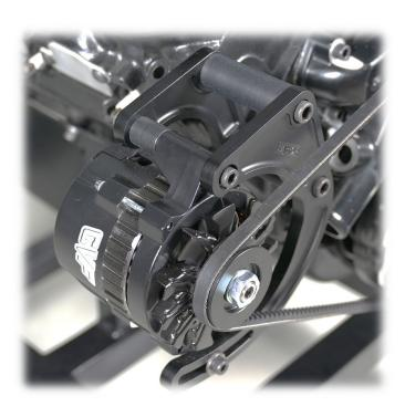
99-ABKT16415 Bracket Asm Alternator BBC (Suits a V-belt GM CS130 140amp Alternator with 6-12 oclock mtg and 6.6" bolt spacing)
