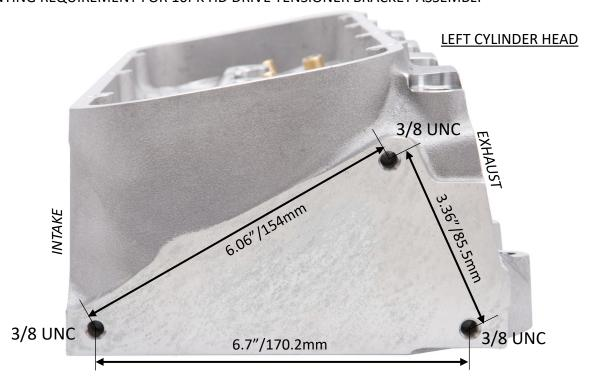
MOUNTING REQUIREMENT FOR OPTIONAL ALTERNATOR MOUNTING KIT - 10PK HD DRIVE
